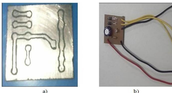
**Figure 3** – a) Board after corrosion and b) Final assembled circuit
