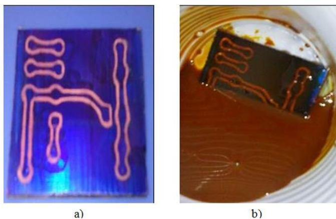
Figure 2 – a) Board after ink application and b) Board submerged at iron perchlorate solution
